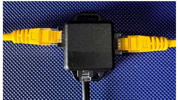
Fig 1 Using the Drop-down Cable, connect the RJ22 port on the Splitter to the MODBUS port on the PDU.
